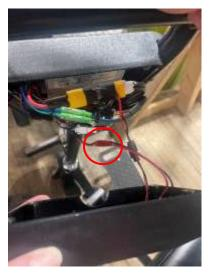
9. Install the wire guide (if your model of scooter does not already have one). Starting on the left side of the wires, insert the guide between the controller box and the controller.
