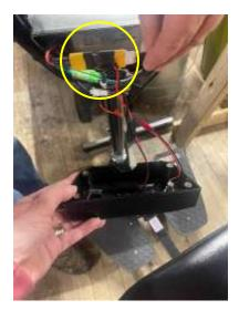
8. Plug in the charge port on the new USB cover. Be sure to align the ridge on the female end (cover side) with the channel on the male end of the red charge port connection.
