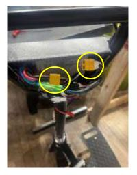
7. Plug in the yellow battery plug connector on both sides on the new USB adapter.
