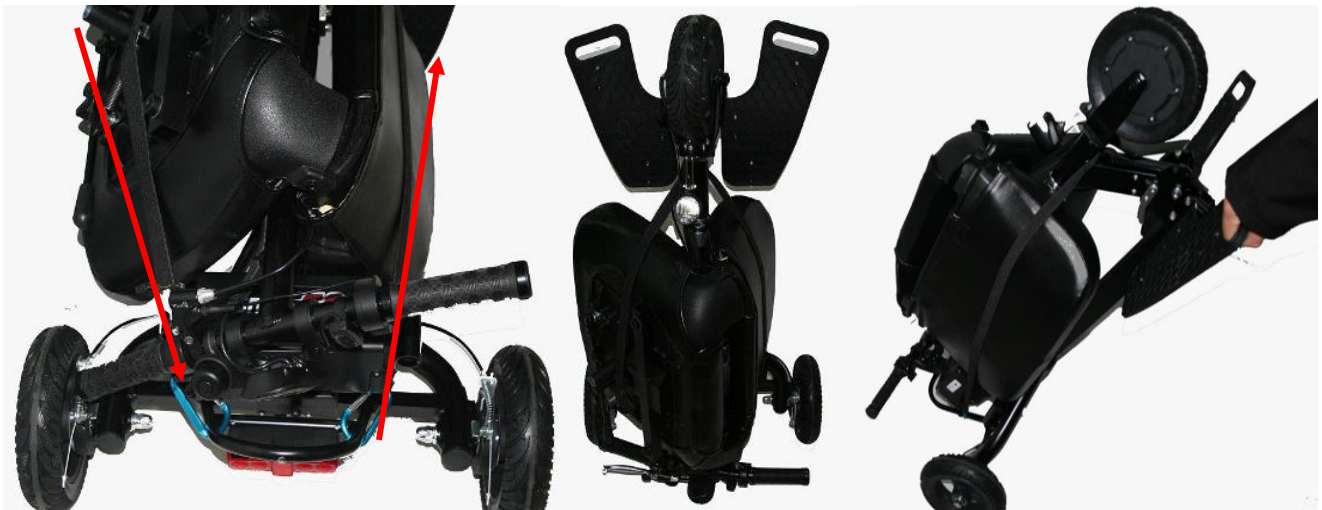
Seat stored on the scooter using the travel bungee.
