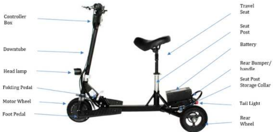
Scooter Side View Unfolded with Travel Seat
